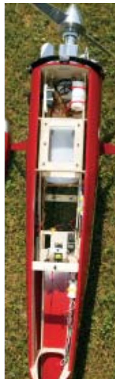
Equipment access doesn't get much easier than this! The entire top of the fuselage lifts off the Waco.
